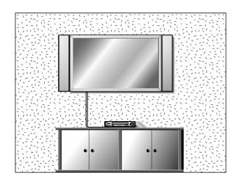
For proper ventilation, allow a clearance of 4" on each side and 2" from the wall. Detailed installation instructions are included from your dealer in the optional Wall Mounting Bracket Installation and Setup Guide.
